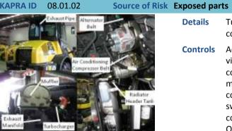
Turbocharger, exhaust manifold, radiator header tank, exhaust pipe, muffler, alternator belt and air conditioning compressor belt.
