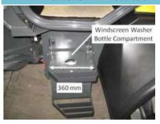
Details Windscreen washer bottle compartment landing width is 360 mm.
