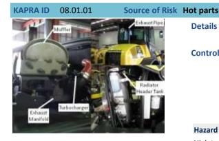
**Details** Turbocharger, exhaust manifold, radiator header tank, exhaust pipe and muffler may become hot during and following operation.
