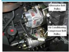
**Details** Air conditioning compressor belt pulley and alternator belt pulley.
