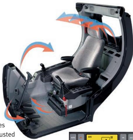
The high performance air conditioning provides an air flow which is adjusted and electronically controlled for the conditions. Five operating modes enable even the most demanding operator to be satisfied.
