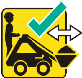
5. TRANSPORT MATERIAL WITH BUCKET DOWN AND LEVEL
