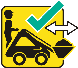
5. TRANSPORT MATERIAL WITH BUCKET DOWN AND LEVEL
