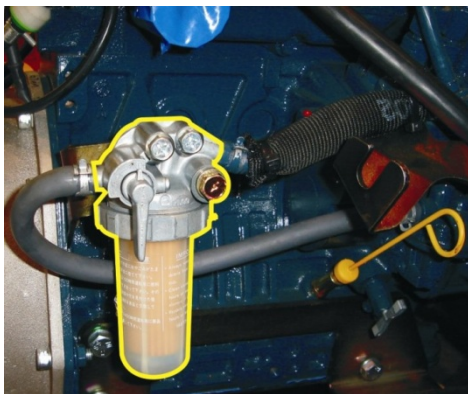
Photo showing early model fuel filter up to March 2008 .
