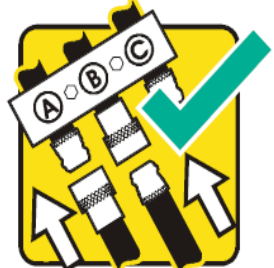
4. ENSURE HYDRAULIC HOSES ARE CLEAN AND ATTACHED
