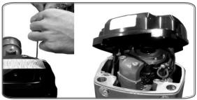
3) Pull the brush spring backwards and remove the brush.
