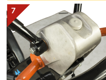
7 LARGE VOLUME OIL TANK
