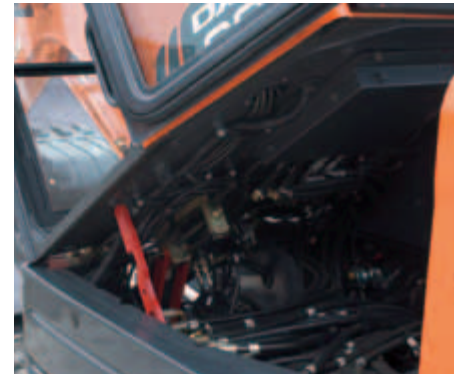
Tilting cabin for easy maintenance
