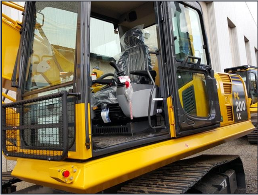
Handrails and grab rails installed.
