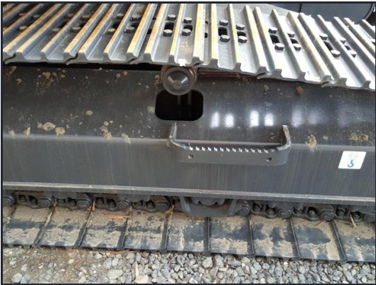
Rung step at cabin access.
