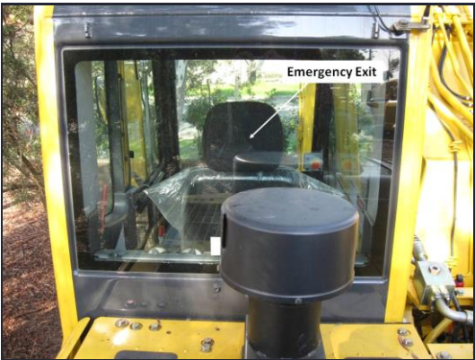
Emergency egress through the back of the cab
