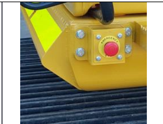
E-stop on front RHS of machine.
