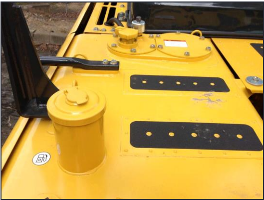
Fuel fill point and top of hydraulic tank
