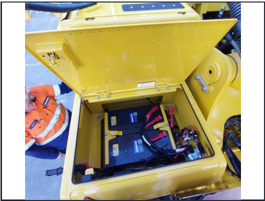
Battery box access.
