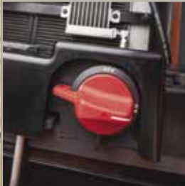
Battery cut-off switch
