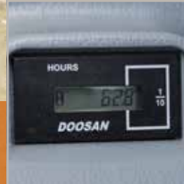
Hour meter (from ground level)
