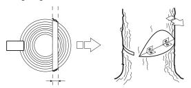
All control over the felling direction is lost if the felling hinge is too narrow or non-existent, or if the directional cuts and felling cut are badly placed.
