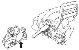
Regularly check that the brake band is at least 0.6 mm thick at its thinnest point.
