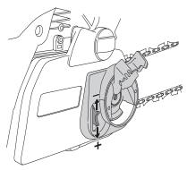
The chain is correctly tensioned when it does not sag from the underside of the bar, but can still be turned easily by hand. Hold up the bar tip and tighten the bar knob by turning the knob clockwise.
