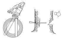
Finish the felling cut parallel with the directional cut line so that the distance between them is at least 1/10 of the
