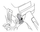
CAUTION! The start/stop switch automatically returns to run position. In order to prevent unintentional starting, the spark plug cap must be removed from the spark plug when assembling, checking and/or performing maintenance.
