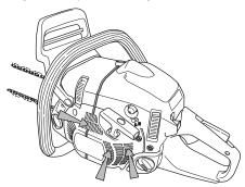
IMPORTANT! In order to maintain operation of the centrifugal cleaning system it must be regularly maintained. Clean the air intake to the starter, the fins on the flywheel, the space around the flywheel, inlet pipe and carburettor compartment.
