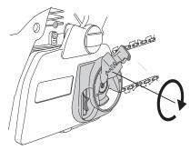
When fitting a new chain, the chain tension has to be checked frequently until the chain is run-in. Check the chain tension regularly. A correctly tensioned chain ensures good cutting performance and long life.
