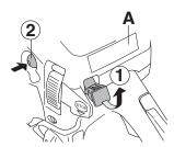
Grip the front handle with your left hand. Hold the chain saw on the ground by placing your right foot through the rear handle. Pull the starter handle with your right hand and pull out the starter cord slowly until you feel a resistance (as the starter pawls engage) then pull firmly and rapidly until the engine fires (3).
