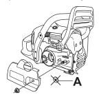
Fit the bar over the bar bolt. Place the bar in its rearmost position. Place the chain over the drive sprocket and in the groove on the bar. Begin on the top side of the bar.
