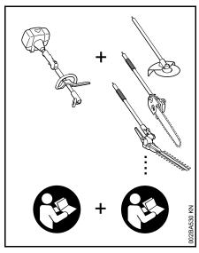
In the STIHL KombiSystem a number of different KombiEngines and KombiTools can be combined to produce a power tool. In this instruction manual the functional unit formed by the KombiEngine and KombiTool is referred to as the power tool.
