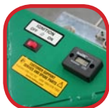
Tachometer shows engine RPM & service intervals
