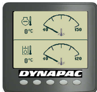
Fig. Temperature screen
