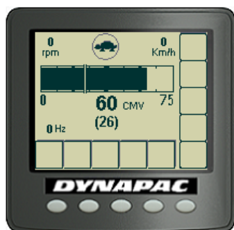
Fig. Compaction meter display (CMV display)
