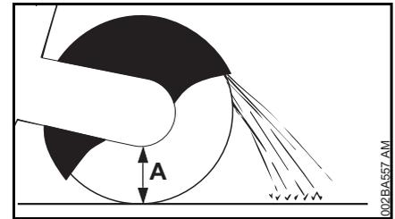
The procedure is dependent on the outer diameter of the pipe and the maximum possible cutting depth of the abrasive wheel (A).
