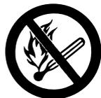
Gasoline is an extremely flammable fuel. If spilled and ignited by a spark or other ignition source, it can cause fire and serious burn injury or property damage. Use extreme caution when handling gasoline or fuel mix. Do not smoke or bring any fire or flame near the fuel or the power tool. Note that combustible fuel vapor may escape from the fuel system.
