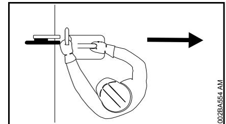
3. Position the cut-off machine in such a way that your body is clear of the cutting attachment. Avoid standing in direct line with the wheel (See illustration.) Never bend over the cutting attachment, especially when the guard is pulled back towards the top and there is a risk of reactive forces. Ensure sufficient freedom of movement, especially in trenches. Make sure there is sufficient space for the user and the fall of the severed part.
