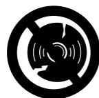
Inspect the abrasive wheel frequently and replace immediately if the abrasive wheel is cracked or warped. Cracked or warped wheels may shatter or break and cause serious or fatal personal injury. Out-of-round or unbalanced abrasive wheels increase vibration and reduce the service life of the cut-off machine.
