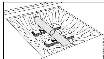
Support an exposed pipe in a trench so that it is stable and capable of bearing weight. If the ends of the pipe are firmly in the ground, the ground may act as a support where the pipe emerges into the open. Additional support will be needed closer to the cut, however, to prevent sagging (see illustration). Be alert for pipe that is under stress that may cause it to shift when cut; pipe in the ground may be under stress because of uneven surfaces.
