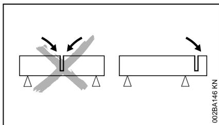
Avoid wedge action. The severed part must not bind the abrasive wheel.
