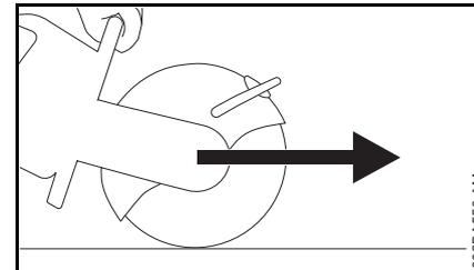
The most common reactive forces are pull-away and climbing. If the contact is at the bottom of the wheel, a cut-off machine will try to pull away from the operator (pull-away.) If the contact is at the front of the wheel, the wheel may attempt to climb the object being cut (climbing.)
