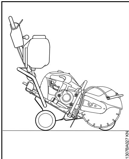
The cut-off machine can be mounted on the STIHL cut-off machine cart FW 20 (special accessory) in a few easy steps.
