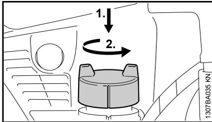
Press the cap down with your hand as far as possible, turn it counterclockwise (approx. 1/8 turn) and remove it.
