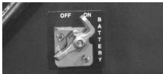
Figure 13.10 - Battery Isolate Switch
