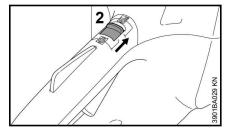
• Unlock the power tool by moving the retaining latch (2) to ♂.
