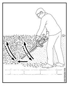
Swing the cutting blade from the bottom upwards in an arc – lower the nose of the blade, move along the hedge and then swing the blade up again in an arc.
