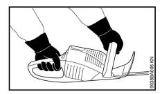
Left hand on the control handle and right hand on the loop handle.
