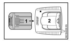
Slide the battery (1) into the charger (2) until you start to feel resistance – then push it in until it engages.
