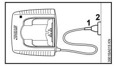
Insert the plug (1) in the wall outlet (2).
