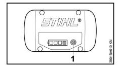
Press button (1) to activate the display – the display goes off automatically after 5 seconds.
