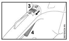
Move the retaining latch (3) to the trigger switch (4) cannot be operated – the power tool is locked to prevent start-up.
