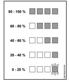
If the LEDs on the battery flash or glow red – see "If the red LEDs glow continuously / flash".
