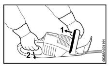
Release the switch lever (1) and the trigger switch (2).
