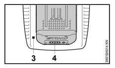
The LED (3) on the charger comes on when the battery is inserted – see "LED on Charger"
