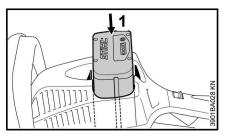
Insert the battery (1) in the power tool – the battery slides into the compartment – press it down carefully until it snaps into position – the battery must be flush with the top of the housing.
