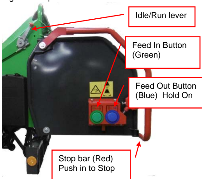
Fig 3.4.1 Stop Bar and Feed control Buttons
