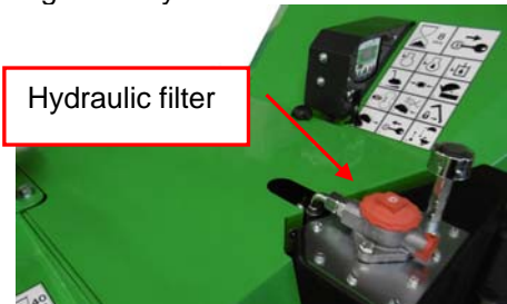
Fig 6.20 Hydraulic Return Filter
