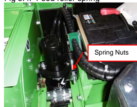
Fig 5.4. Feed roller spring
