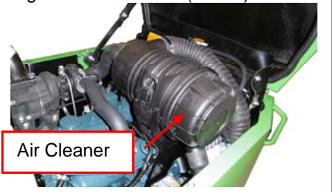
Fig 6.11 Air Cleaner (Diesel)
