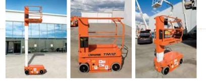
The Snorkel TM12 provides a safe, efficient means of working at height in restricted spaces typically encountered in offices, retail stores, hotels, public buildings or crowded industrial aisles. Its ultra compact size makes it ideal for applications such as stock picking and record storage retrieval. When the job is complete, the lift can be quickly lowered and returned to a convenient storage area.
