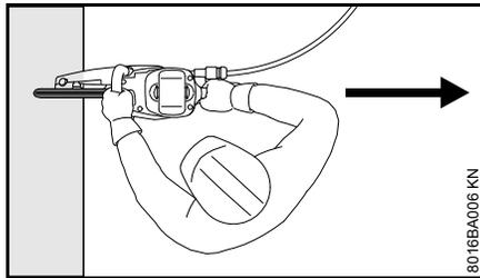
Do not stand in line with the abrasive wheel. Ensure sufficient freedom of movement, especially in construction trenches there must be sufficient space for the user and for the part being cut to fall.
