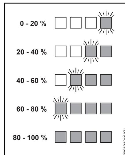
The LEDs on the battery go off automatically when the charge process is completed.
