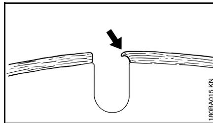
If work continues with dull segments, these may soften due to the high heat generated – the parent wheel is annealed and its strength is compromised – this can lead to stresses that are clearly recognizable by gyrations of the abrasive wheel. Do not continue to use the abrasive wheel – **Risk of accident!**
