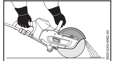
Set the abrasive cutting wheel guard so that particles of material are guided away from the user and cut-off machine.
