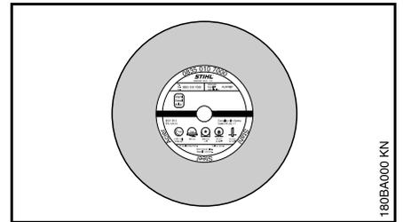
Composite resin abrasive wheels are also known as bound abrasive wheels.
