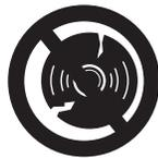
Frequently inspect the abrasive cutting wheel – replace it right away if there are visible cracks, buckling or other damage (for example, overheating) – **risk of accident due to breakage!**
