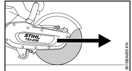
The cut-off machine pulls forward, away from the user, when the abrasive cutting wheel touches the object to be cut from above.
