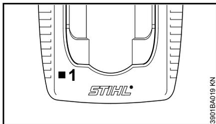
A self test is performed after the charger is connected to the power supply. During this process, the light emitting diode (1) on the charger lights up green for about 1 second, then red and goes off again.
