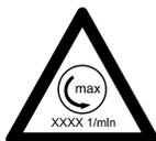
The permissible speed of the abrasive cutting wheel must be equal to or greater than the maximum spindle speed of the cut-off machine. – Refer to the chapter "Specifications".
