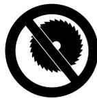
Never use circular saw blades, carbide, rescue or wood cutting attachments or saws of any kind – **these may cause fatal injuries!** Instead of uniformly removing particles as when cutting with an abrasive wheel, the teeth of a circular saw blade may snag in the material. This causes the cut-off machine to react in a highly aggressive manner with uncontrolled and extremely dangerous kickback.
