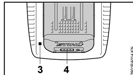
The LED (3) on the charger comes on when the battery is inserted – see "LED on Charger"
