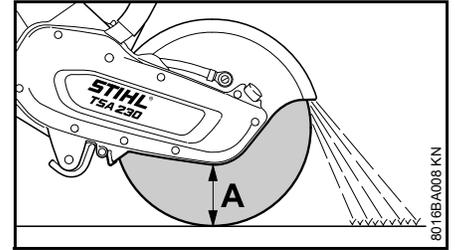
The procedure is dependent on the outer diameter of the pipe and the maximum possible cutting depth of the abrasive cutting wheel (A).
