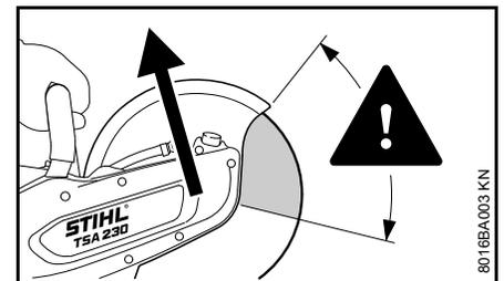
Kickback occurs when the cut-off machine is suddenly thrown up and back in an uncontrolled arc towards the operator.
