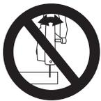
The abrasive wheel must be guided straight in the cut, without wedging. Never exert lateral pressure on the abrasive wheel.
