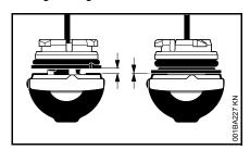
Left: Base of cap in closed position (with open space)
