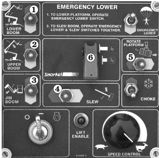
Figure 7.22 - Platform Control Switches
