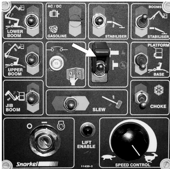
Figure 2.1 - Emergency Stop Switch at Ground Control Box
