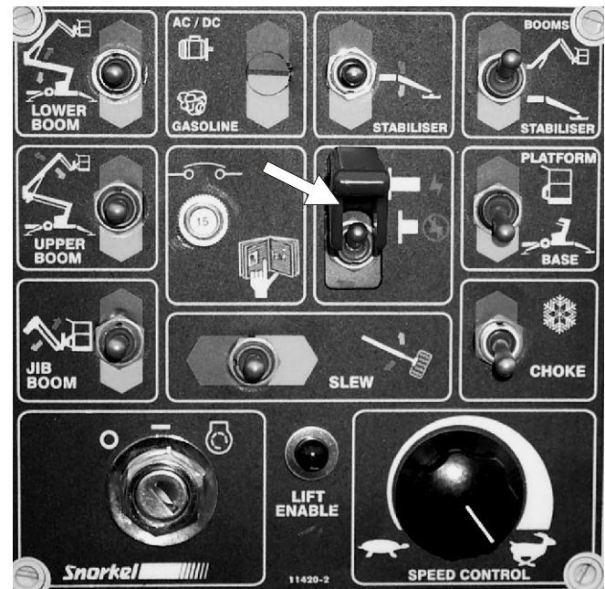
Figure 8.1 - Ground Control Box Emergency Stop Switch Location.
