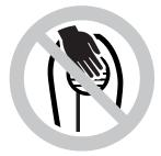
The machine may overheat if the cooling air inlet is covered. This can cause serious damage to the machine and/or the operator. Never block or cover the cooling air inlet.
