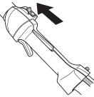
Start the engine and make sure the engine stops when you move the stop switch to the stop setting.
