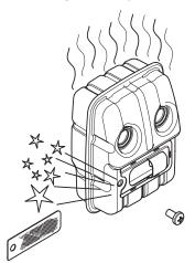
**CAUTION!** Never use a machine with a defective muffler.
