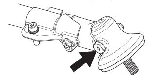
The grease in the bevel gear does not normally need to be changed except if repairs are carried out.
