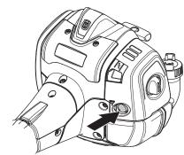
Choke: Move choke control up to choke position.
