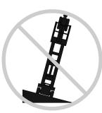
Do not depend on the tilt alarm as a level indicator. The tilt alarm sounds on the chassis and in the platform when the machine is on a severe slope.
