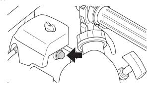
Choke: Set the choke control in the choke position.
