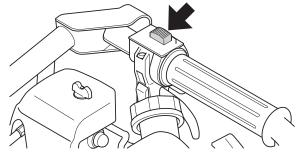
Start the engine and make sure the engine stops when you move the stop switch to the stop setting.
