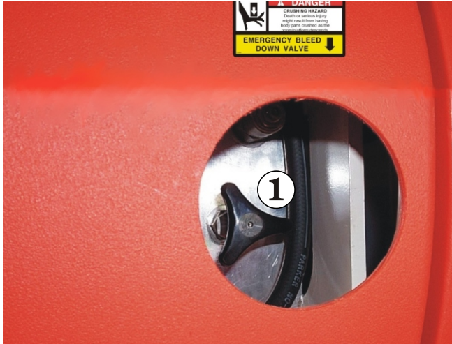
Figure 9.5 - Manual Lower Valve
