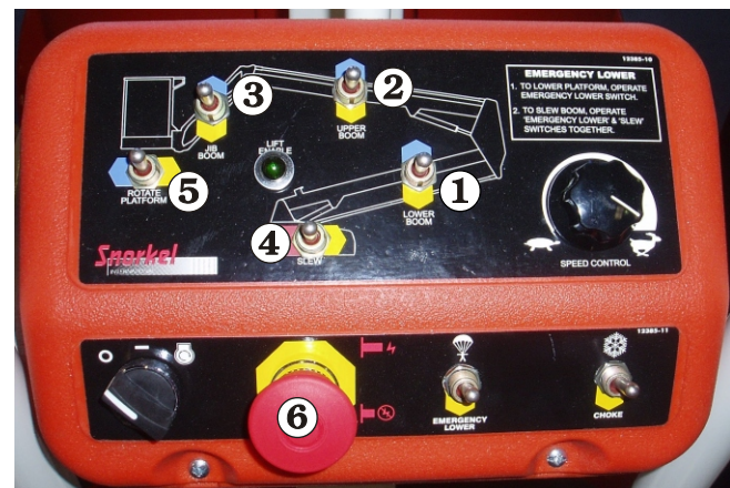
Figure 7.24 - Platform Control Switches
