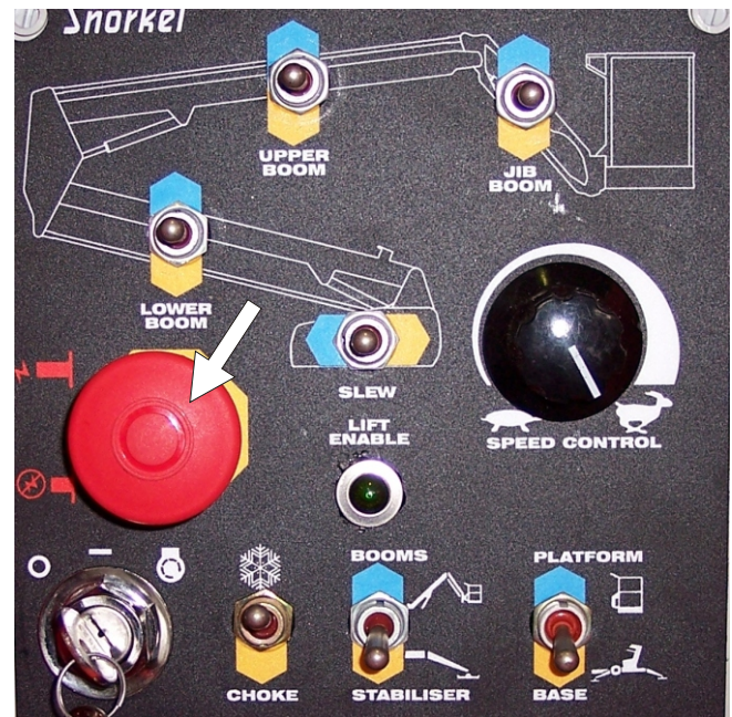
Figure 8.1 - Ground Control Box Emergency Stop Switch Location.
