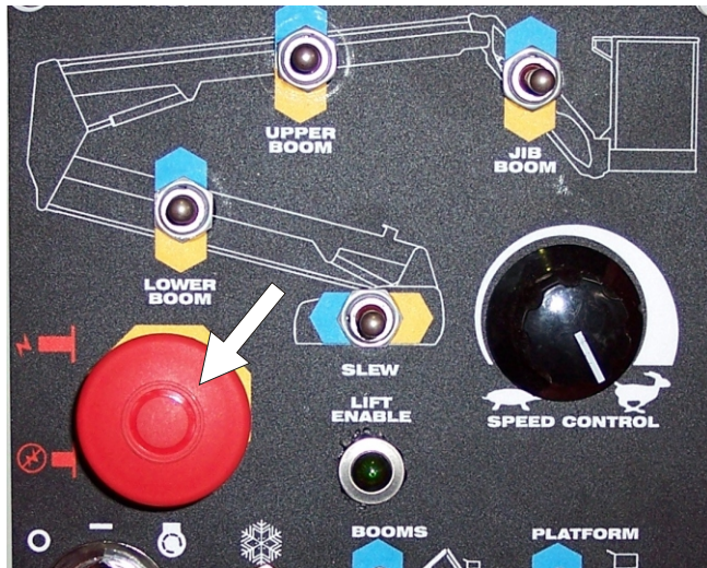
Figure 2.1 - Emergency Stop Switch at Ground Control Box
