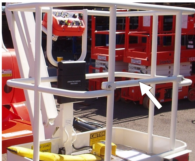
Figure 7.19 - Platform Gravity Gate
