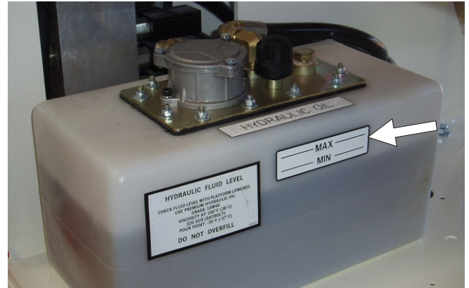
Figure 4.3 - Hydraulic Oil Level
