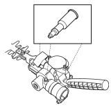
CAUTION! The gear housing must not be filled completely with grease. The grease expands as the machine heats up during operation. If the gear housing was completely filled with grease it could damage the seals and lead to leakage of grease.
