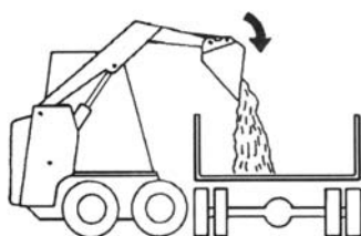
Fig. 19: Dumping Into a Box
