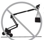
Do not place or attach fixed or overhanging loads to any part of this machine.
