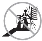
Be aware of crushing hazards when grasping the platform guard rail.
