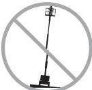
Do not depend on the tilt alarm as a level indicator. The tilt alarm sounds in the platform only when the machine is on a severe slope.
