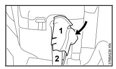
Push the throttle cable support (1) on to the handle (2) from the side and engage in position
