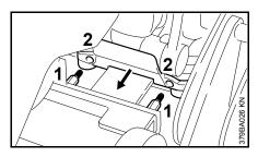
Position the cut-off machine so that the pins (1) protrude into the holes in the support (2)
