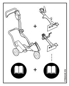
A basic machine **and** an attachment kit are combined to produce a complete cart FW 20.
