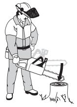
When the bar hits the stump the brake should be applied.
