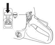
The engine is stopped by pushing the stop switch to the stop position.
