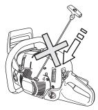
Note! Reactivate the chain brake by pushing the front hand guard back towards the front handle. The chain saw is now ready for use.
