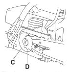
The front hand guard is not designed solely to activate the chain brake. Another important feature is that it reduces the risk of your left hand hitting the chain if you lose grip of the front handle.
