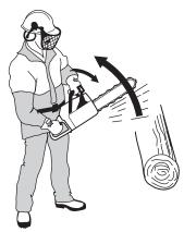
If the kickback is less violent or the kickback zone of the bar is closer to you the chain brake will be activated manually by the movement of your left hand.
