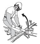
Have control over the workpiece. If the pieces you intend to cut are small and light, they can jam in the saw chain and be thrown towards you. Even if this does not need to be a danger, you may be surprised and lose control of the saw. Never saw stacked logs or branches without first separating them. Only saw one log or one piece at a time. Remove the cut pieces to keep your working area safe.
