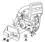
Fit the bar over the bar bolts. Place the bar in its rearmost position. Place the chain over the drive sprocket locate it in the groove on the bar. Begin on the top edge of the bar.
