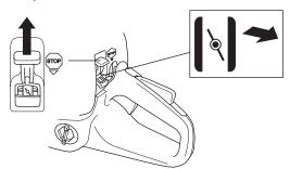
**Start throttle:** The correct choke/start throttle setting is obtained by moving the control to the choke position.
