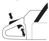
Start the chain saw and apply full throttle. Release the throttle control and check that the chain stops and remains stationary. If the chain rotates when the throttle control is in the idle position you should check the carburettor idle adjustment.
