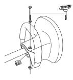
6 Now make a final adjustment to give yourself a comfortable working position. Tighten the screw. CAUTION! The loop handle and hand guard must not be fitted behind the arrow marked on the shaft.
