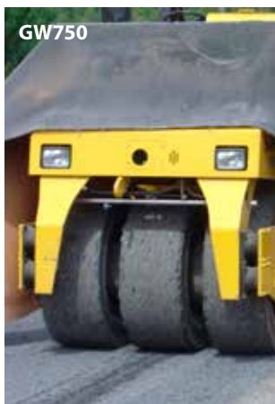
Fig 2. Chip seal pavement finished by GW750
