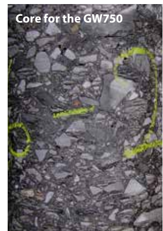
Fig 5. Uniform compaction throughout thick lift ( 27 cm with 3.8cm aggregate size ) HMA pavement layer by two different rollers
