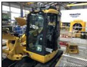
Cabin windows and beacon lighting
