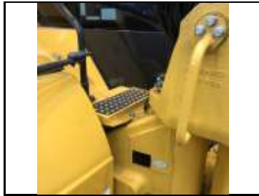
Step 2 on RHS maintenance access
