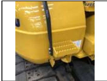
Step 1 on RHS maintenance access
