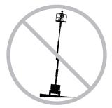
If the tilt alarm sounds while the boom is lowered: Do not extend, rotate or raise the boom above horizontal. Move the machine to a firm, level surface before raising the platform.
