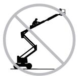
Do not enter or exit the platform unless the machine is in the stowed position and the platform is at ground level.
