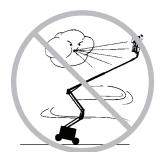
Do not raise the boom when wind speeds may exceed 12.5 m/s. If wind speeds exceed 12.5 m/s when the boom is raised, lower the boom and do not continue to operate the machine.
