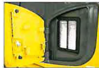
External air conditioner filter
