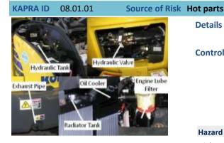
**Details** Exhaust pipe, hydraulic tank, hydraulic valving, engine lube filter, radiator header tank and oil cooler may become hot during and following operation.
