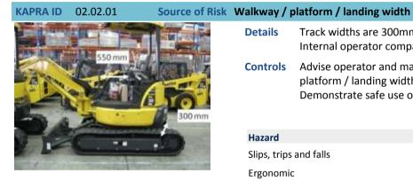
DetailsTrack widths are 300mm.<br/>Internal operator compartment access width / clearance is 550 mm.ControlsAdvise operator and maintenance staff of the potential slips, trips and falls and ergonomics hazards due to walkways /
