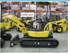
**Details** Interior operator compartment height is 1500mm.
