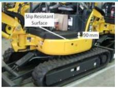
**Details** 90mm variation in floor height at operator compartment entry.
