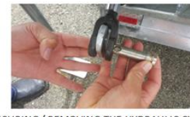
SECURING / REMOVING THE HYDRAULIC CYLINDER TO STOWAGE BRACKET WITH CLEVIS PIN FIG E
