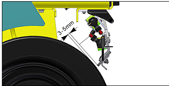
Fig. 9-24 Clearance of scraper to pneumatic wheels
