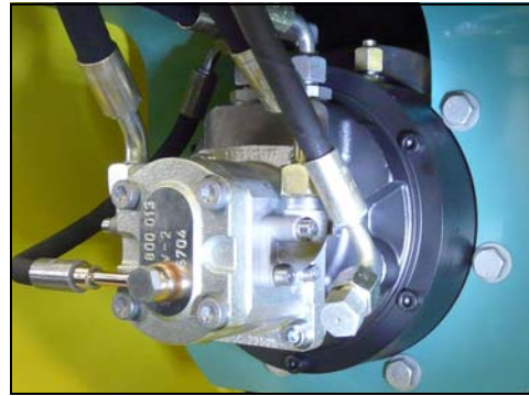
Fig. 9-29 Remove the brake hose and seal it so that it can be pressurized.
