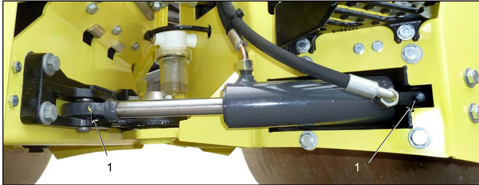
Fig. 9-32 Location of grease nipples on steering cylinder
