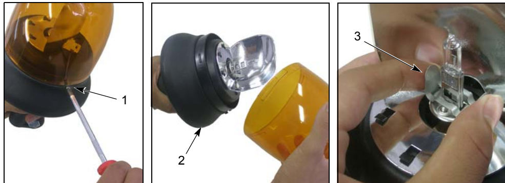
Fig. 8-5 Replacing the bulb
