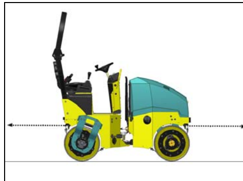
Fig. 9-1 Tow the roller using the towing lugs
