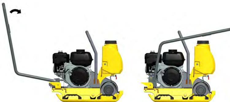
During loading and transport, the control handle must be folded down.
