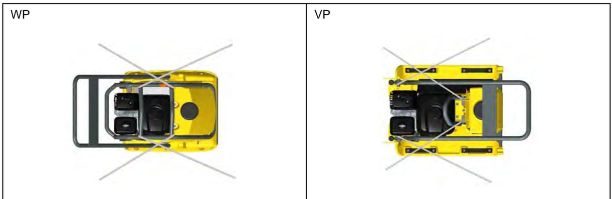
3. After loading the machine, lash down the machine to prevent it from rolling off, slipping, or tipping over. Attach tie-down lugs to the designated lashing points.
