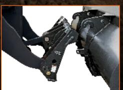
Optional Quick Coupler Quickly change many of your wheel loader's non-hydraulic attachments without leaving the seat. A four-point style pick-up means you can hook up attachments easily, even on irregular terrain.
