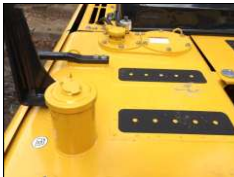
Fuel fill point, hydraulic tank cover & fill point.
