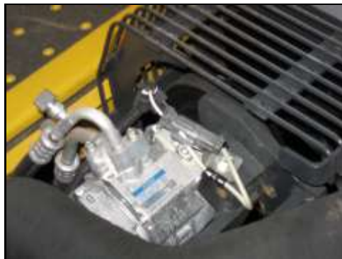
Air conditioning compressor.
