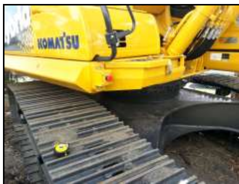
Track step to maintenance access step 1 distance.
