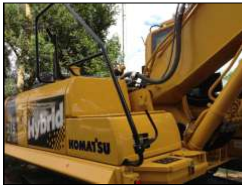
Handrail height of access system.
