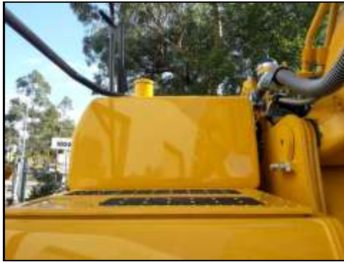
Maintenance access step 2 to top platform distance.
