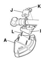
Remove the mounting plate (H). Fit the adapter (I) and bracket (J) with the two screws (K) as shown. Fit the blade guard (A) to the adapter using the 4 screws (L) as shown.
