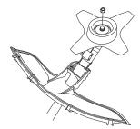
When fitting, tighten the nut in the opposite direction to the direction of rotation of the cutting attachment. To remove it, undo the nut in the same direction as the cutting attachment rotates. (CAUTION! The nut has a left-hand thread.) Tighten the nut using the socket spanner.
