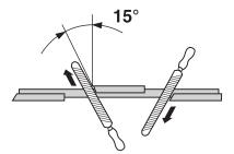
· Adjust the blade setting. This should be 1 mm.
