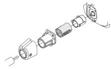
Regularly check the vibration damping units for cracks or deformation.
