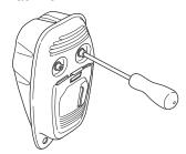
If the muffler on your machine is fitted with a spark arrestor screen this must be cleaned regularly. A blocked screen will cause the engine to overheat and may lead to serious damage.
