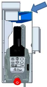
Ultrasonic sensor on the platform controller bracket
