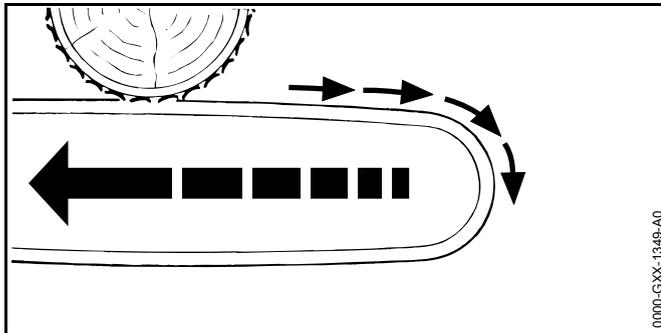
The saw is pushed back toward the operator when the top of the bar is used for cutting.
