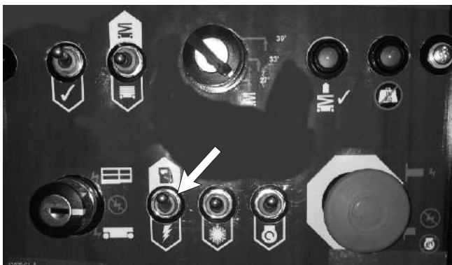
Figure 11.2 - Diesel/Electric Selection Switch
