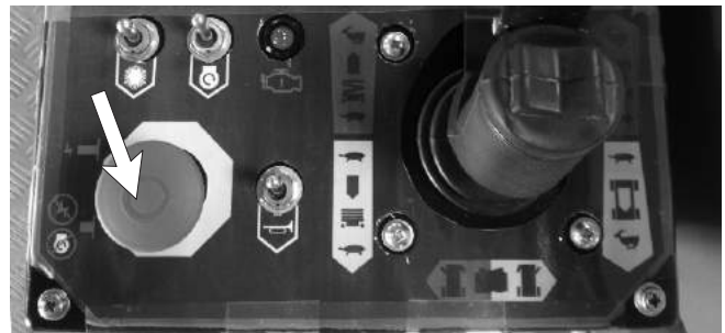
Figure 8.2 - Emergency Stop Switch at Platform Control Box
