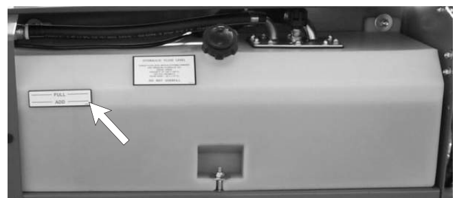
Figure 4.4 - Hydraulic Oil Level
