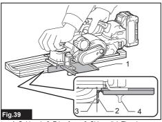
▶ 1. Guide rule 2. Edge fence 3. Side wall 4. Thumb screw
