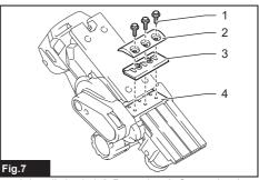
■ 1. Installation bolt 2. Drum plate 3. Conventional planer blade (with adjusting plate) 4. Drum
