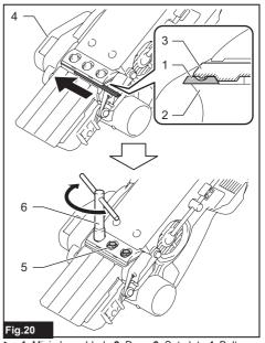
■ 1. Mini planer blade 2. Drum 3. Set plate 4. Belt cover 5. Installation bolt 6. Box wrench
