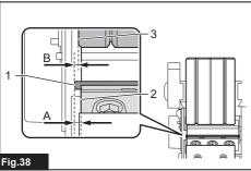
▶ 1. Blade edge 2. Side end of drum 3. Side end of front base
