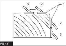
1. Edge fences 2. Small chamfering 3. Large chamfering
