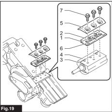
1. Positioning guide 2. Adjusting plate 3. Guide groove 4. Drum 5. Drum plate 6. Set plate
