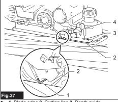
▶ 1. Blade edge 2. Cutting line 3. Depth guide
