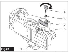
▶ 1. Belt cover 2. Depth guide 3. Washer 4. Thumb screw 5. Mounting hole
