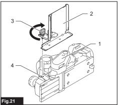
■ 1. Belt cover 2. Guide rule 3. Thumb screw 4. Mounting hole
