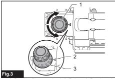
▶ 1. Depth adjustment knob 2. Pointer 3. Depth scale
