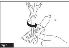
1. Screws 2. Conventional planer blade 3. Adjusting plate
