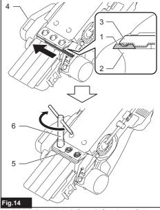
Mini planer blade 2. Drum 3. Set plate 4. Belt cover 5. Installation bolt 6. Box wrench
