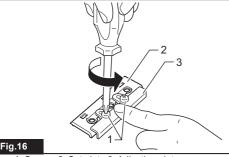
▶ 1. Screws 2. Set plate 3. Adjusting plate
