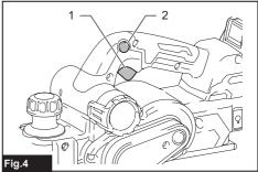
▶ 1. Switch trigger 2. Lock-off button
