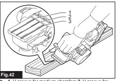
1. V groove for medium chamfers 2. V groove for small chamfers 3. V groove for large chamfers
