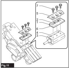
1. Positioning guide 2. Adjusting plate 3. Guide groove 4. Drum 5. Drum plate 6. Conventional planer blade 7. Installation bolt
