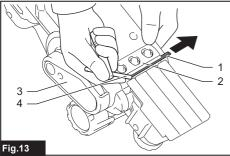
1. Mini planer blade 2. Drum 3. Belt cover 4. T-handle of box wrench
