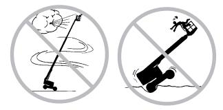
Use extreme care and slow speeds while driving the machine in the stowed position across uneven terrain, debris, unstable or slippery surfaces and near holes and drop-offs. Do not drive the machine on or near uneven terrain, unstable surfaces or other hazardous conditions with the boom raised or extended.
