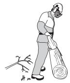
Keep the trunk between you and the chain saw as you move along the trunk.
