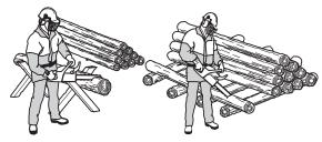
The log is lying on the ground. There is little risk of the chain jamming or the object splitting. However there is a risk that the chain will touch the ground when you finish the cut.
