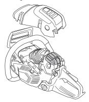
The filter can be cleaned more thoroughly by washing it in water and detergent.
