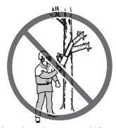
In order to keep control of your saw, always maintain a firm foothold. Never work on a ladder, in a tree or on any other insecure support.
