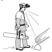
5 Take great care when cutting a tree that is under tension. A tree that is under tension may spring back to its normal position before or after being cut. If you position yourself incorrectly or make the cut in the wrong place the tree may hit you or the machine and cause you to lose control. Both situations can cause serious personal injury.
