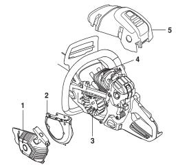
Clean the cooling system with a brush once a week, more often in demanding conditions. A dirty or blocked cooling system results in the machine overheating which causes damage to the piston and cylinder.
