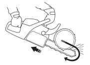
8 Unless the user resists this pushing force there is a risk that the chain saw will move so far backwards that only the kickback zone of the bar is in contact with the tree, which can lead to a kickback.
