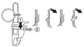
The directional cuts should run 1/4 of the diameter through the trunk and the angle between the top cut and bottom cut should be  $45^{\circ}$ .
