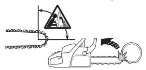
Kickback always occurs in the cutting plane of the bar. Normally the chain saw and bar are thrown backwards and upwards towards the user. However, the chain saw may move in a different direction depending on the way it
