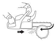
9 Follow the instructions on sharpening and maintaining your bar and chain. When you replace the bar and chain use only combinations that are recommended by us. See instructions under the headings Cutting equipment and Technical data.
