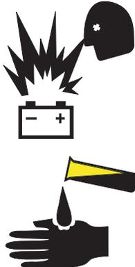
Batteries contain acid. Always wear protective clothing and eye wear when working with batteries.
