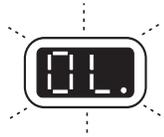
Flashing OL in the LED diagnostic readout indicates the platform is overloaded and no functions will operate. An alarm will sound.
