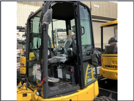
Grab rail installed.
